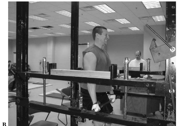
FIGURE 2. Isometric mid-thigh clean pull testing apparatus. (A) schematic of apparatus setup; (B) photo of testing apparatus setup.
